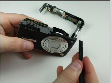
Using the spudger, pry off the top cover by gliding the spudger along the entire edge between the top cover and the front cover.
