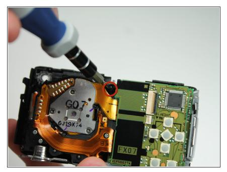
Remove the small screw in the hole towards the top of the camera(#00P, 5.4mm).
