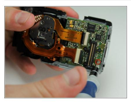
Remove the small screw holding down the lower motherboard(#00P, 3.2mm).
