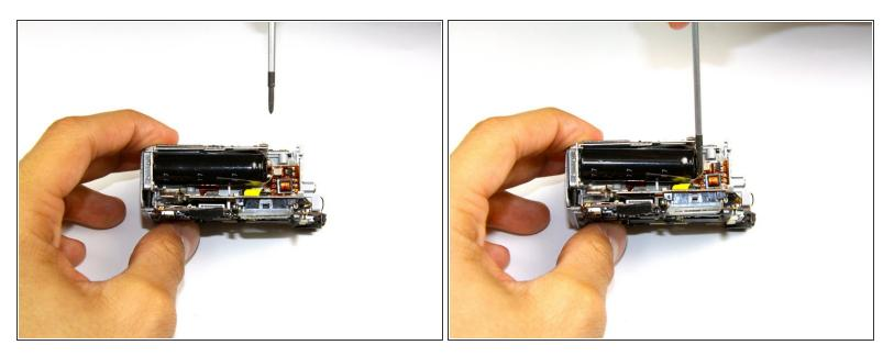
Caution: the capacitor, a black cylinder near the top of the camera, might have a charge in it, which could be harmful to you or the camera. Neutralize it by touching both wires with a screwdriver at the same time.
