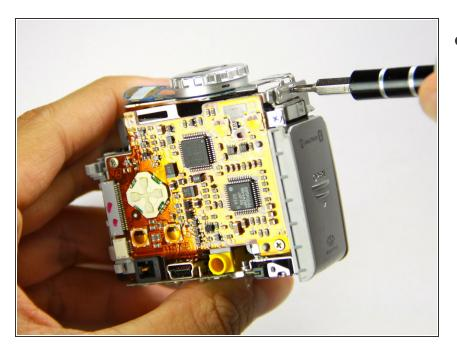
Remove the 3.0mm Phillips #000 screw at the top of the battery door.
