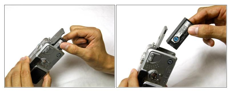
• Remove the battery from the camera.
