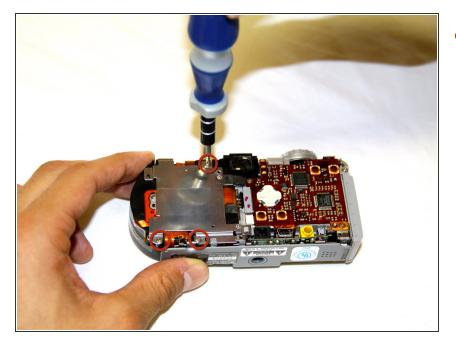
Remove the three 4.0mm Phillips #000 screws holding the back panel in place.
