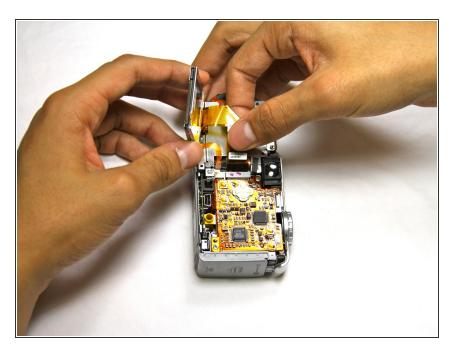
• Pull the two ribbon cables out of their slots on the back circuit board.
