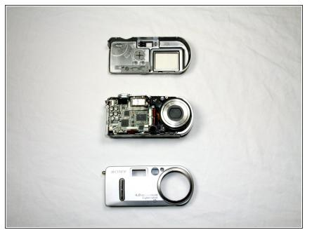
• After the casing is removed, the camera should look as shown.
