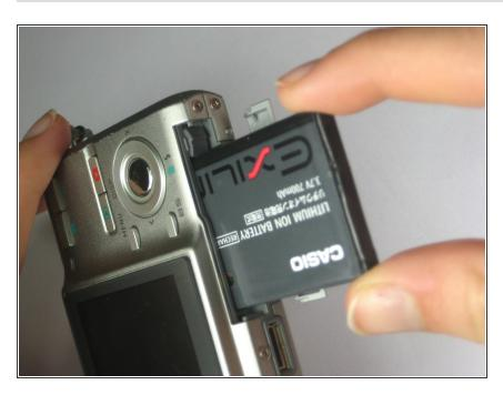
Firmly grasp each side of the battery and pull it out of its compartment.
