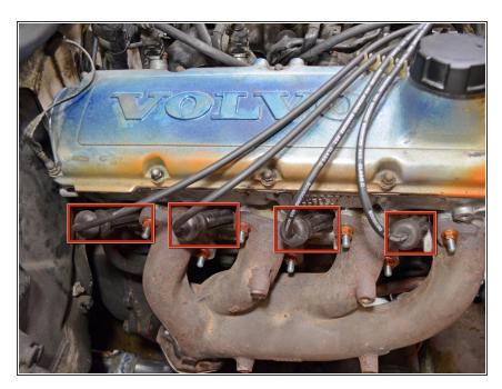
The four spark plugs are located on the passenger side of the engine near the exhaust manifold. Replace the spark plugs one at a time.
