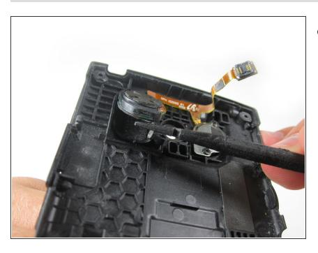
Use the flat edge of the spudger to gently pry and remove the speaker.
