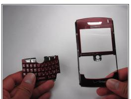
Remove the keyboard from the front casing.
