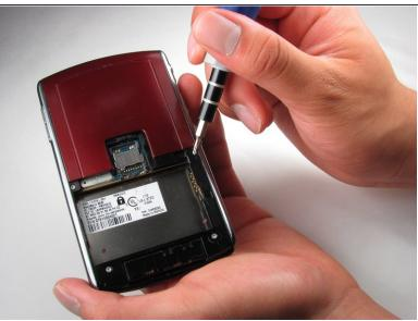
Once the battery is removed, remove the four 9.2 mm screws with the T4 Torx Screwdriver.
