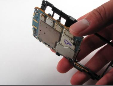
With the motherboard revealed, slowly lift it off of the casing.
