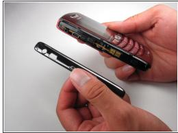
Remove side panels with the Plastic Opening Tool by sliding it along the edge of the panel until you can pry it off with the tool.
