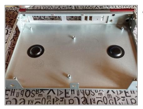
The rubbers prevent the plate from contacting the chassis.
