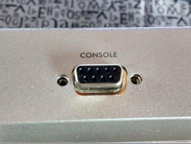
To remove the cover it is necessary to disconnect the DB9 connector
