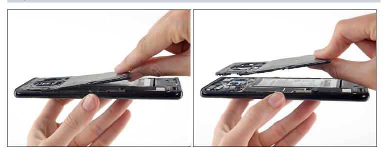
• Remove the NFC antenna and charging coil assembly.
