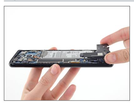
• Remove the loudspeaker assembly.
