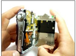
• Carefully pry the top portion of the screen from the camera.
