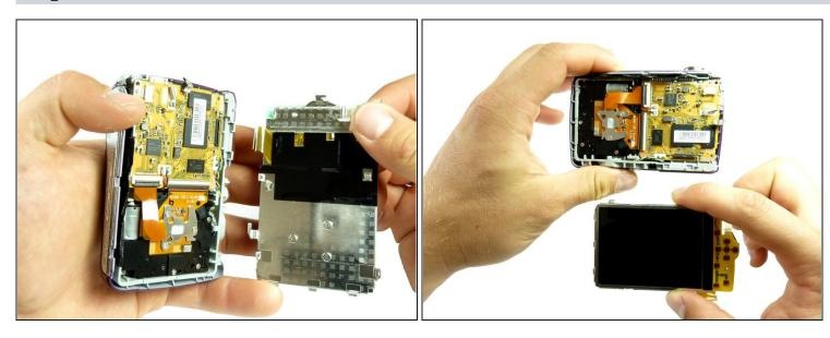
• The LCD screen is now completely removed from the rest of the camera.
