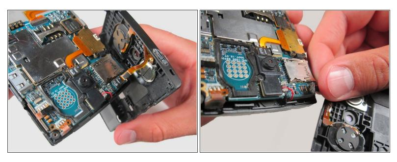
Slowly remove the back casing by gently pulling the ribbon connection.
