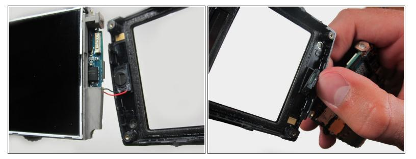
Gently pull on the wires to remove the front casing.
