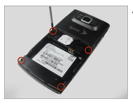
Using the Phillips #00 screwdriver, remove the four indicated screws (4.5 mm).
