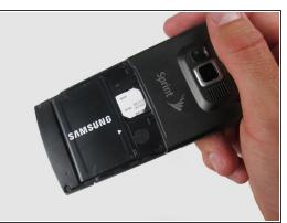
To remove the back casing, firmly press down and push towards the bottom of the phone.
