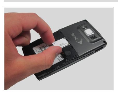
To remove the SIM card, start by pressing the top of the card and push down and away towards the bottom of the phone. Then, as indicated, pull the SIM card out.
