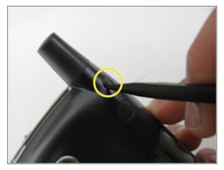
• Using the spudger, remove the small rubberized patch under the antenna.
