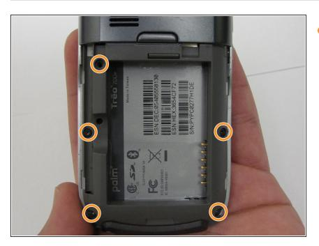
After removing the battery and stylus, unscrew the 5 Torx screws (using a T-5 Torx screw driver)
