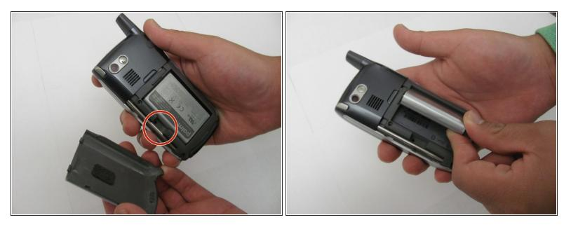
• Use the small notch on the left hand side of the phone to remove the battery.
