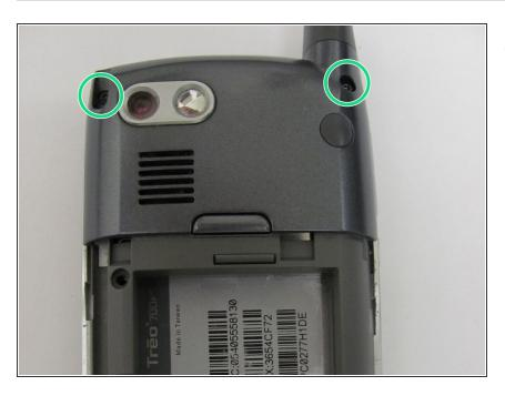
Unscrew the last two screws using the previous screw driver.
