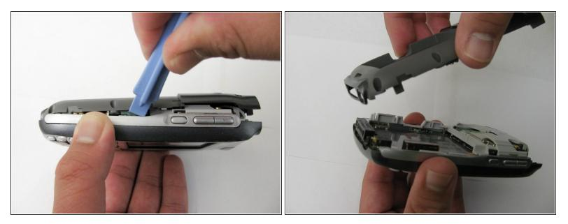
• Using the plastic opening tool, gently separate the back case from the phone body.
