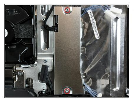
Remove the two T10 Torx screws securing the inverter to the rear case.
