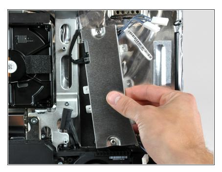
• Pull the inverter away from the chassis and lift it slightly out the rear case.
