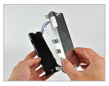
• Lift the metal case off the inverter.
