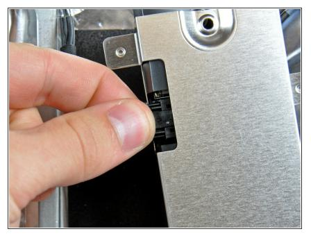
Disconnect the inverter cable by simultaneously squeezing the locking mechanism and pulling the connector away from its socket.
