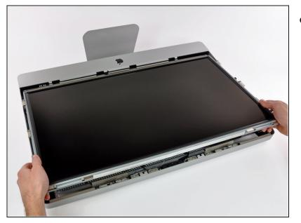
• Carefully pull the display toward the top edge of your iMac and lift it out of the outer case.
