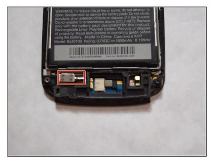
The component denoted in the red box is the vibration motor. Remove the component by desoldering the surface-mount joints.
