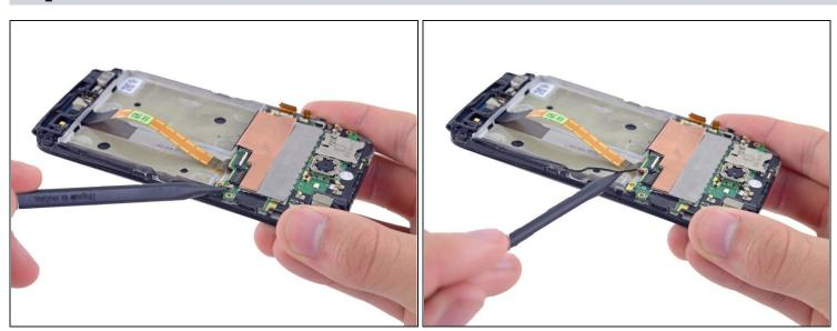
• Using the pointed end of the spudger, pop the antenna cable from its connector on the motherboard.
