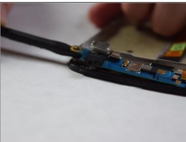
• Using the nylon spudger, remove the circuit board from the phone.
