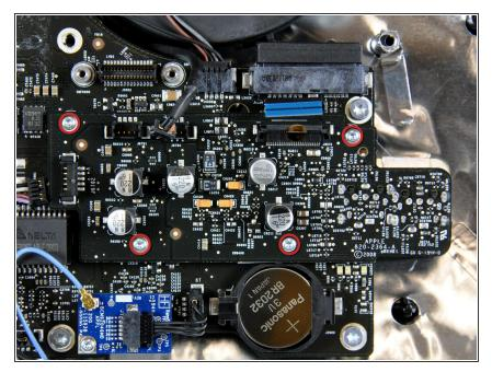
Remove the four T6 Torx screws securing the audio board to the logic board.
