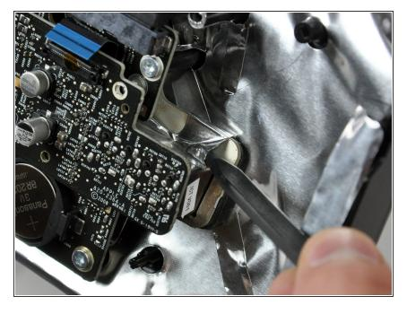
Use the sharp end of a spudger to remove the EMI aluminum tape covering the microphone/headphone jacks.
