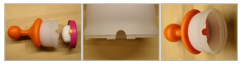
• The lamp opens up at the base: there are two smaller tabs next to the button, the semi-transparent plasic can be pressed in a bit with a knife, put a bit of paper inbetween to prevent the clip from snapping back. Next go with a knife towards one of the large tabs on the side until one side snaps out. Repeat for other side.
