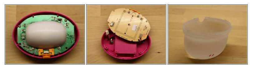
• Remove the 4 screws (warning: 2x2 different types), out comes the pcb. Detach battery connector at the back.
