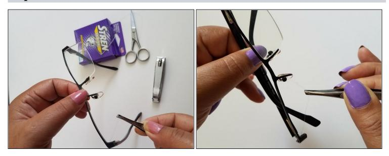
• Remove the old wire/string from the spectacles using the <u>tweezers</u> as shown in the pictures to the right.
