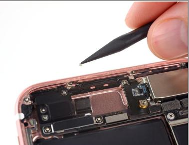
• Use the tip of your spudger to remove any remaining smaller bits of adhesive.
