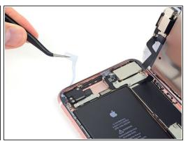
While supporting the display, use tweezers to begin peeling off the final release liners, exposing the adhesive.
