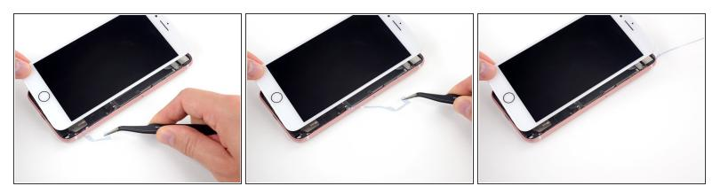
Hold the display out of the way as you remove the final piece of release liner.
