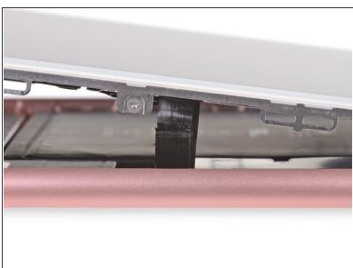
Before closing up the display, check to make sure that all cables are clear.
