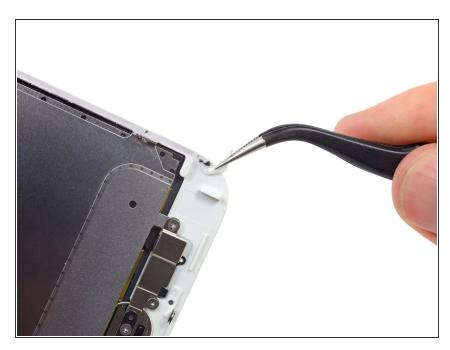
If you're reinstalling your existing display rather than replacing it with a new one, be sure to remove any remaining adhesive from the back of your display as well.
