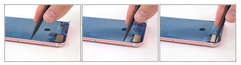
Use the tip of a spudger to press all the adhesive into place around the entire perimeter of your iPhone.
