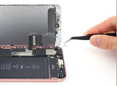
i The release liner may consist of two or more pieces. As you remove the final piece, you may need to pause and reposition the display.
