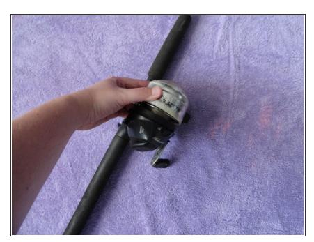
Grab onto the cap of the reel and begin to unscrew it from the base, turning it in a counter-clockwise direction. This will expose the mechanism and line inside.
