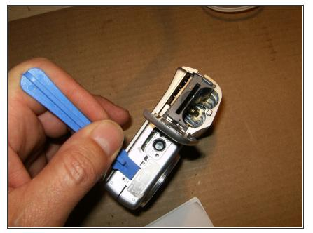
• Open the battery cover and split the housing carefully. Start at the battery compartment and work your way around it. You can use an opening tool or your fingernails. Also make sure to open the USB port cover.
