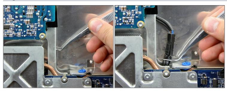
• Use a pair of tweezers to pull the AC-in cable out from underneath the chassis.
