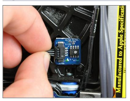
Disconnect the hard drive thermal sensor by pulling the connector away from its socket parallel to the face of the hard drive.
