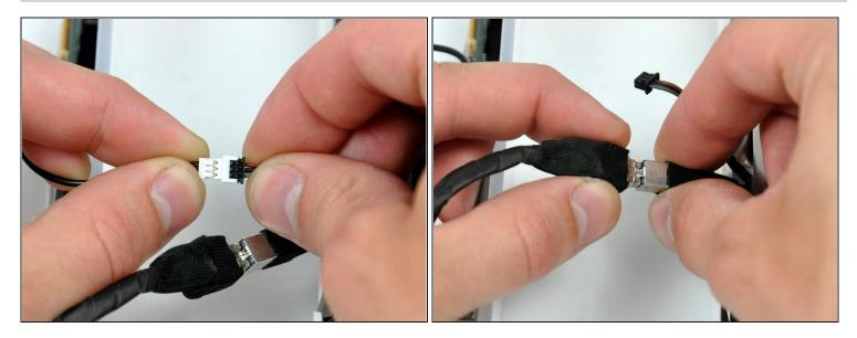
• Disconnect both the camera and microphone cables.
