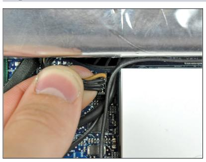
Pull the inverter cable connector up off its socket on the logic board.
