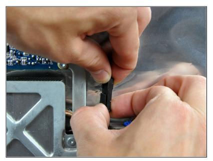
Disconnect the AC-in cable by depressing the lock mechanism while pulling the connector away from its socket.
