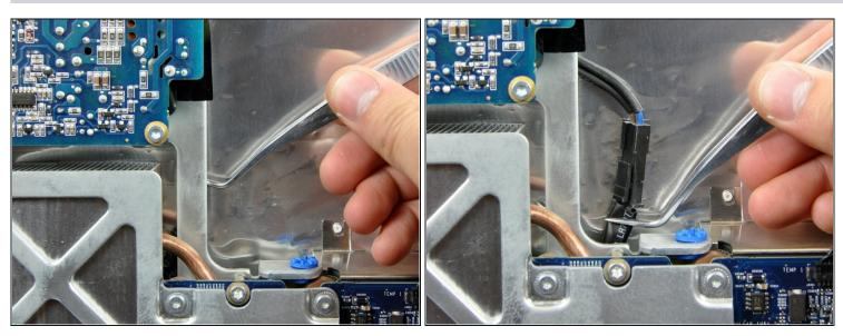
• Use a pair of <u>tweezers</u> to pull the AC-in cable out from underneath the chassis.
