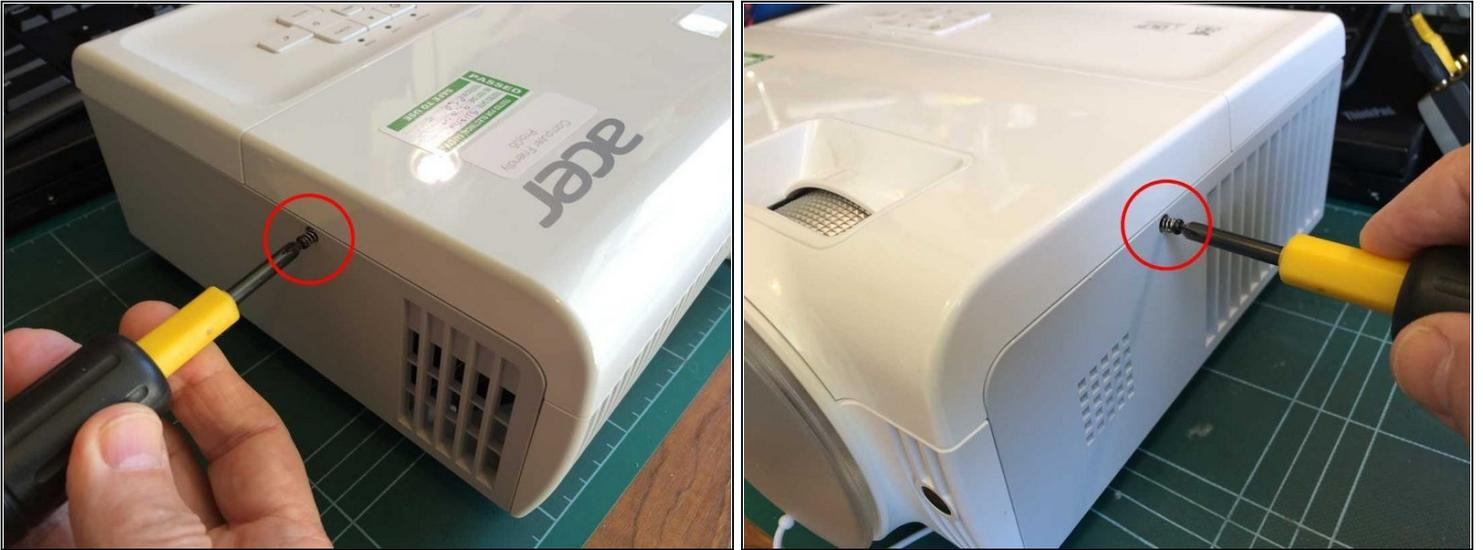
**⚠ The bulb gets extremely hot. To avoid danger of burns, do not start disassembly until the projector has been switched off and allowed to cool for at least 30 - 40 minutes.**
