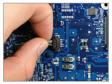
• Disconnect the hard drive fan connector from the logic board by pulling it straight away from its socket.
