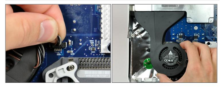
• Disconnect the CPU fan connector from the logic board by pulling it straight up from its socket.
