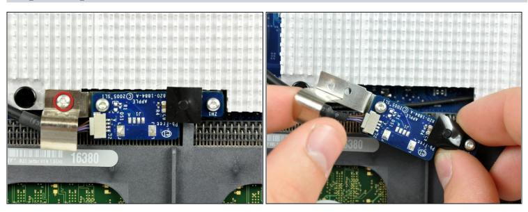
• Remove the single 5 mm T6 Torx screw securing the IR board bracket to the logic board.
