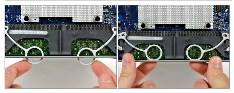
• Push the two RAM arms protruding from the access door inward and set them on the lower edge of the rear case to prevent them from getting caught when removing the logic board.
