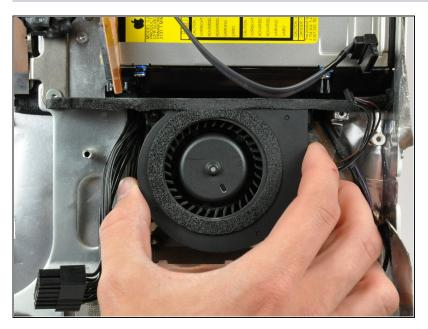
• Lift the optical drive fan off the plastic posts protruding from the rear case.
