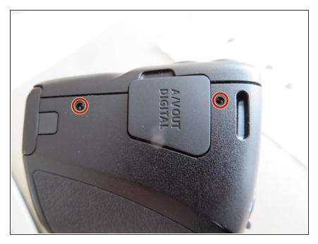
Remove both screws near the A/V out
