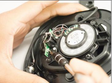
Remove the two 2 mm long screws securing the motherboard using a Phillips #000 screwdriver.
