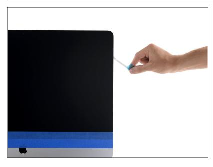
• Repeat the previous steps to remove the protective films from all the remaining adhesive strips.
