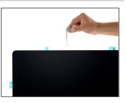
• Remove the protective film from strip 01 by pulling its tab straight up.
