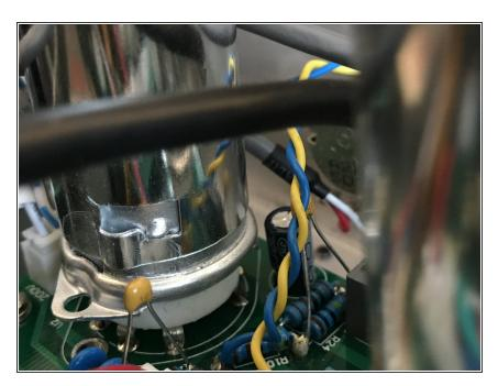
The tubes are covered by a metal shield. To remove this shield, push down a bit and rotate, then pull up the shield.
