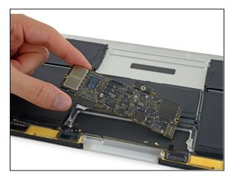
• Remove the logic board.
