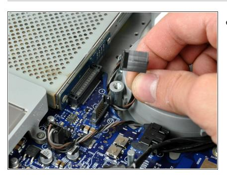
De-route the fan cable from around the edge of the logic board as necessary.
