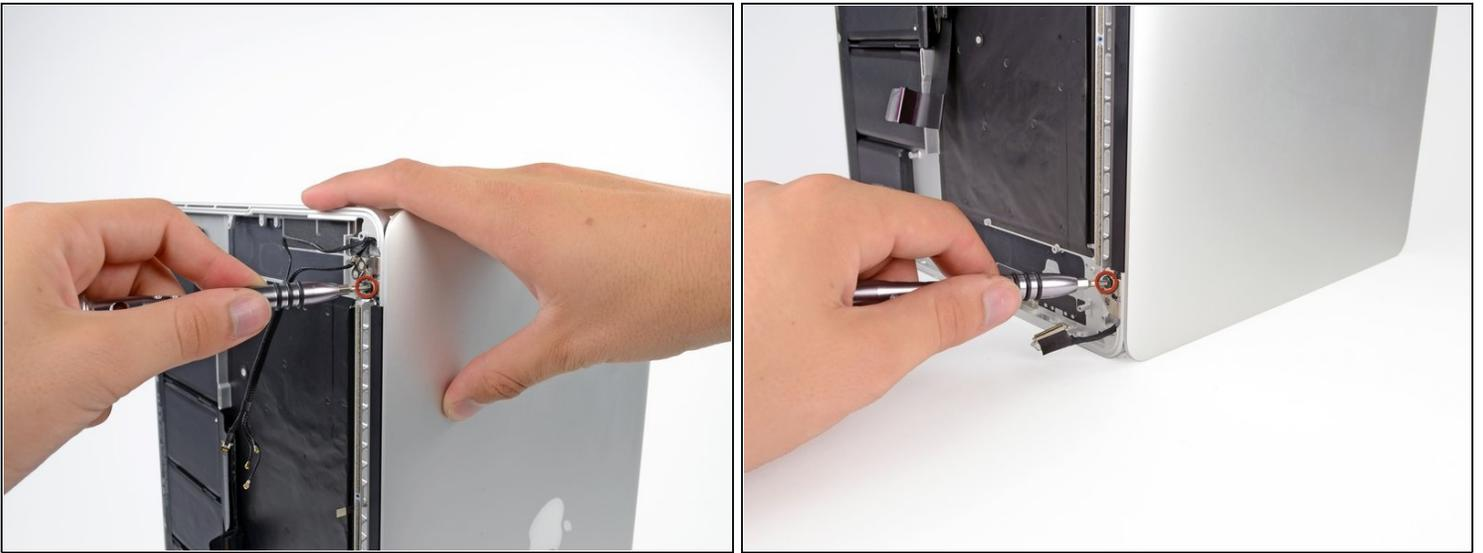
ⓘ Open the device between 90 and 100 degrees, then rest it on its side.
