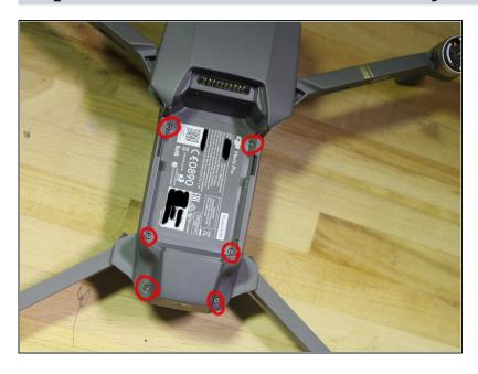
• There are 6 screws on the top of the drone. Four of them are located under the battery, and the other two are right on the back end of the drone. They are all 5.8mm long, and have a 1.5mm hex head, I, however, found that they are easier to remove using a T6H Torx bit.
