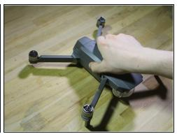
• To start removing screws, you must first remove the battery, by squeezing the sides of the battery, as shown in the photos, and lighting it up and away from the drone.
