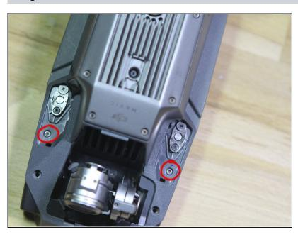
There are two 1.5mm hex screws, these are 5.8mm long, with a 2mm diameter. These are thicker than the screws holding the covers down, because those screws are only holding the covers down, while the screws under it are holding the top cover down. Take note of this during reassembly.
