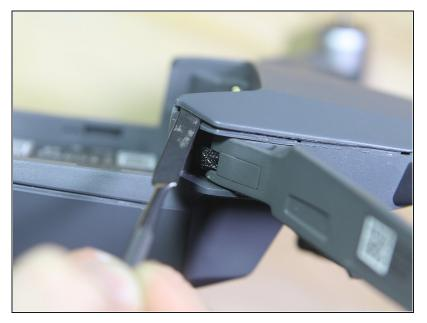
Insert your metal spudger in between the top and bottom case on both the left and right sides of the drone, as shown in the photo. Pry up gently until it is free.
