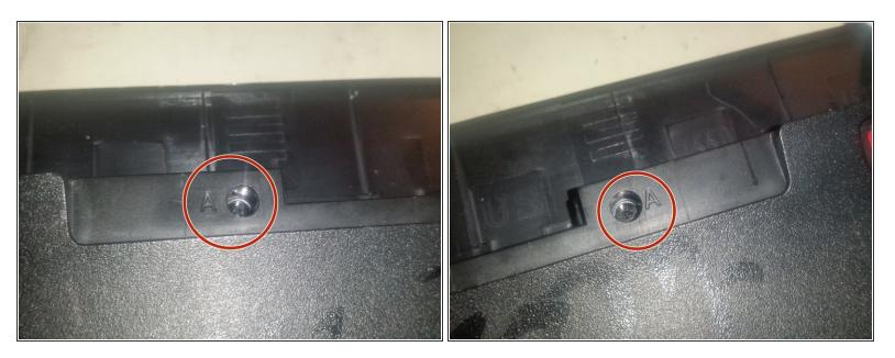
• Remove the two additional short screws from under where the battery was.
