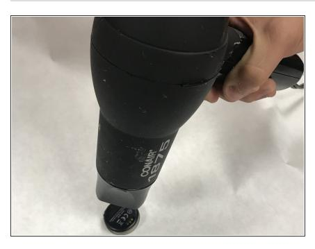
Lightly heat device with hair dryer for 15 seconds to soften adhesive.
