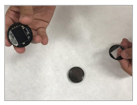
Remove polymer cover that is protecting the mother board, it should just come out when two halves are separated.
