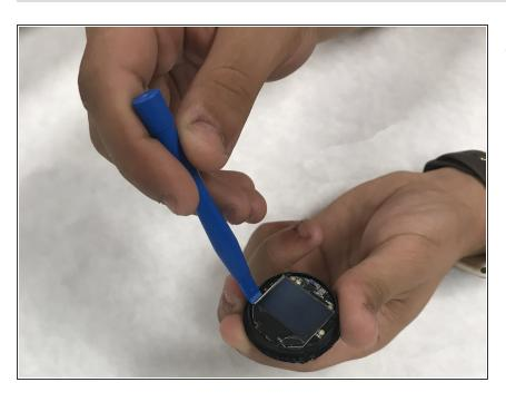
Use a spudger or plastic opening tool to assist the removal of the motherboard. Pry up on two tabs and the mother board will pop out.
