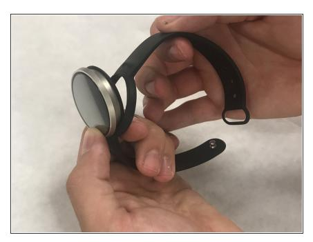
Pull the elastic band away from the device as shown. You will need to use one hand to support the device and pull the elastic band with the other at about a 45 degree angle.
