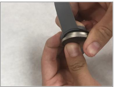
Place the elastic band into the channel in the side of the device shown in the picture. The band will
