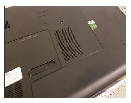
Simply slide the lever to the opposite position, and then the battery will rise upward. Grab it and pull it out.
