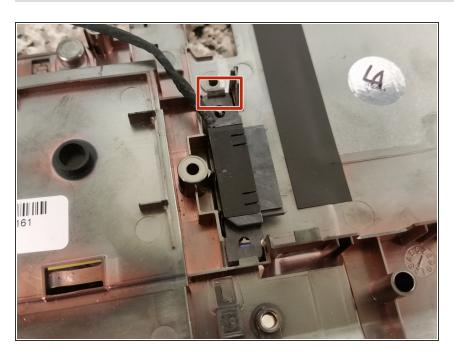
Pull on the clip for the optical drive connector, and then pull the connector out.
