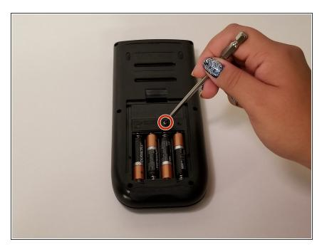
Unscrew the Phillips screw on the internal battery cover.
