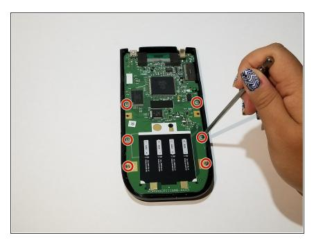
Remove the six Phillips head screws from the circuit board.
