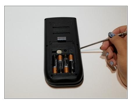
Using a spudger or similar prying tool carefully pop the back of the calculator off.
