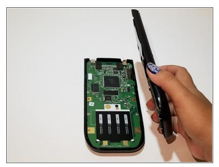
Remove the back of the calculator.
