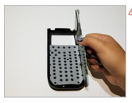
Remove the circuit board and the attached display screen. Make sure not to damage the circuit board.
