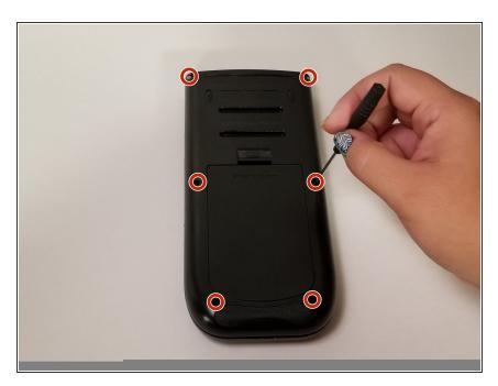
Remove the six T6 screws from the back of the calculator.
