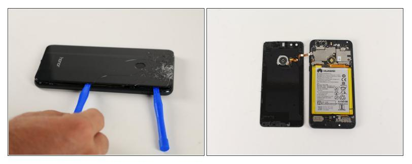
$\bigwedge$  Be careful not to tear the orange ribbon wire when removing the back panel.
