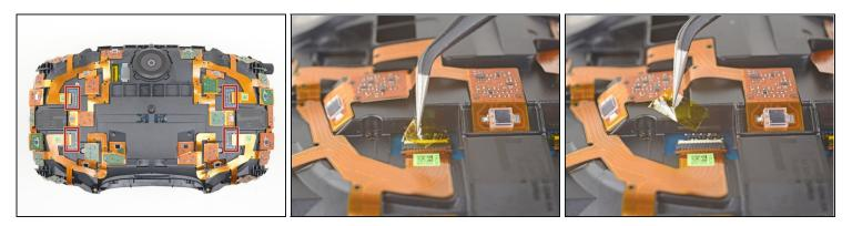
• Use <u>tweezers</u> to remove the clear tape over all four of the sensor array cable connectors.
