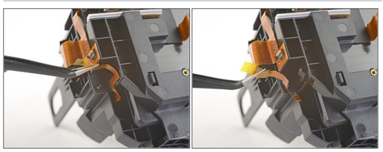
• Gently peel the eyepiece midframe cable off of the facerest midframe.
