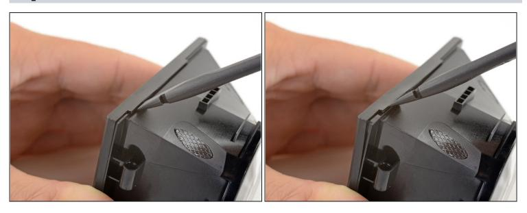
• Use the flat end of a spudger push up one edge of the OLED cover and start unclipping that edge.
