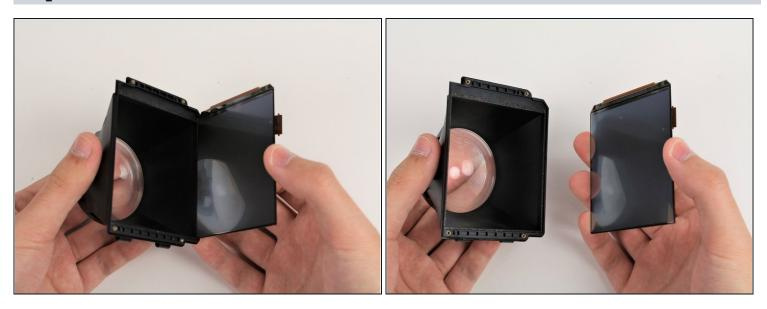
• Remove the screen from the eyepiece housing by pulling the two pieces away from each other.
