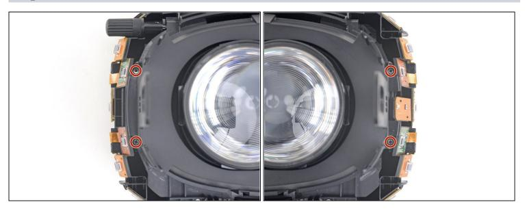
Use a PH000 driver to remove the four 3.9 mm screws securing the sensor array.
