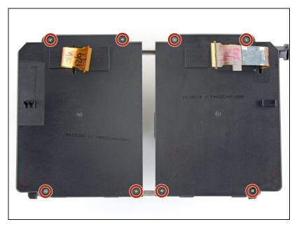
• Use a PH000 driver to remove the eight 2.4 mm screws securing the OLED covers.
