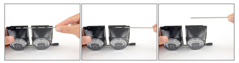
• Slide the support rod out of its brackets on the lens and OLED frames.
