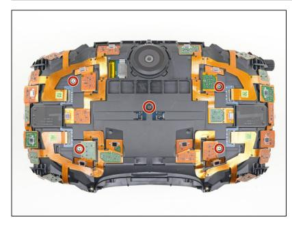
• Use a PH000 driver to remove the five 3.9 mm screws securing the sensor array.
