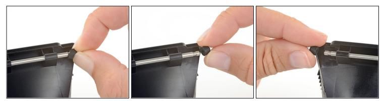
• Pull the rubber bumpers off of either end of the support rod.
