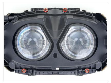
Use a PH000 driver to remove the four 3.9 mm screws securing the facerest midframe.
