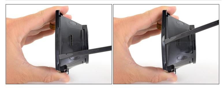
• Slide the spudger under the clip along that edge to free the rest of the edge.
