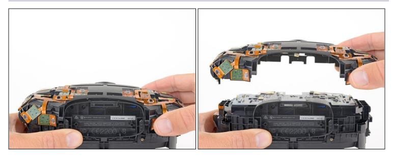
• Lift the sensor array away from the headset to remove it.
