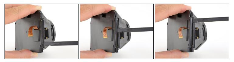
• Slide the spudger around the remaining edges of the OLED cover to unclip those edges.
