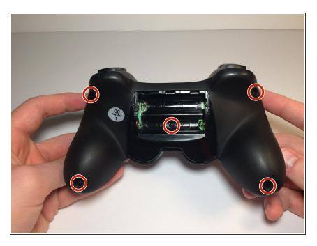
Remove the five screws from the back of the controller using the #0 Phillips screwdriver.
