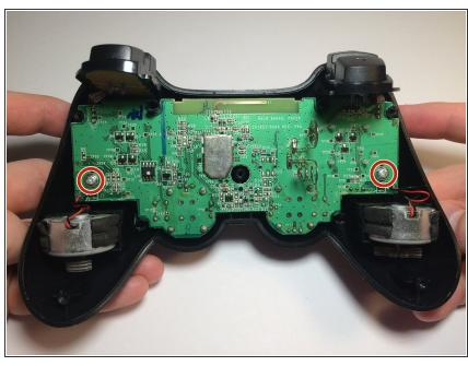
Remove the two screws from the motherboard using the #0 Phillips screwdriver.
