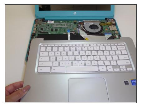
Lift the keyboard panel up and away from the CPU, completely revealing the mainframe.
