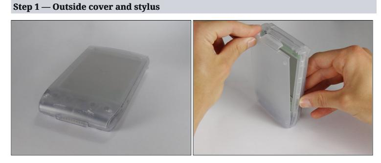
Remove the outer screen cover by releasing the top clip from the main body of the device.
