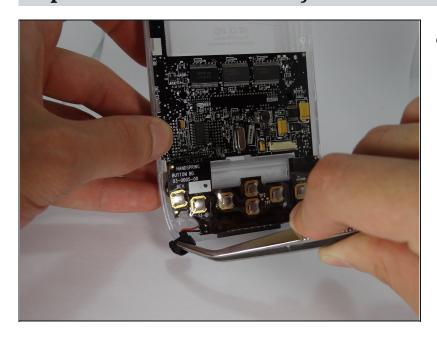
• Use <u>tweezers</u> to remove the power button from the back case.
