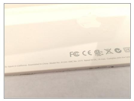
The underside of the keyboard is affixed by a layer of adhesive that covers the entire surface. There are no screws holding the rear cover in place.
