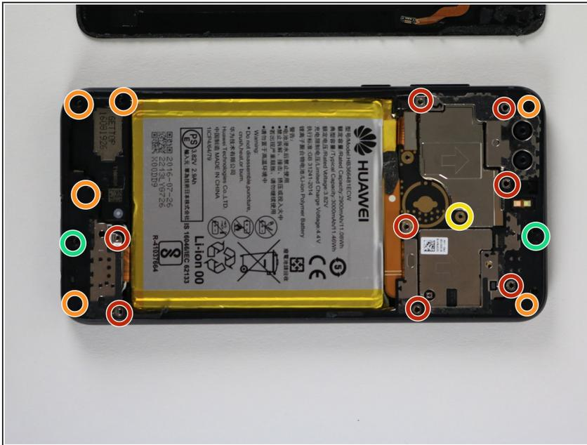
**i** Keep the tiny screws on a magnetic pad or a designated area so they will not be lost. There are eighteen screws in total.
