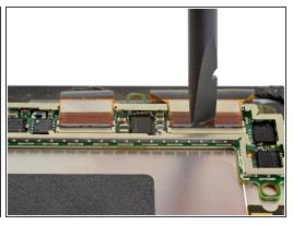
Use a spudger to flip up the small locking flaps on the display cable ZIF connectors.
