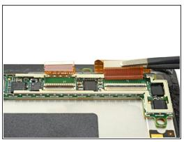
Use tweezers to slide the display cables straight out of their sockets on the display board.
