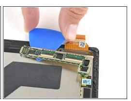
Slide an opening pick under the display board to separate the adhesive holding it onto the back of the screen.
