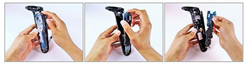
• Lift the motherboard up and out of the Vive controller using your hands.
