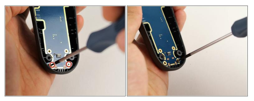
Use the T5 Torx screwdriver to remove the two silver 4.2mm screws from the bottom of the motherboard.
