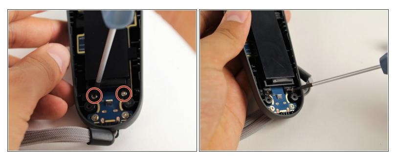
Use the T5 Torx screwdriver to remove the two silver 4.2mm screws from the bottom of the battery frame.
