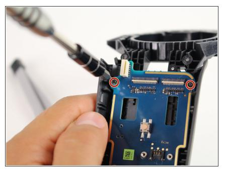
Use the Phillips 00 screwdriver to remove the two black 5.8mm screws from the top of the motherboard.
