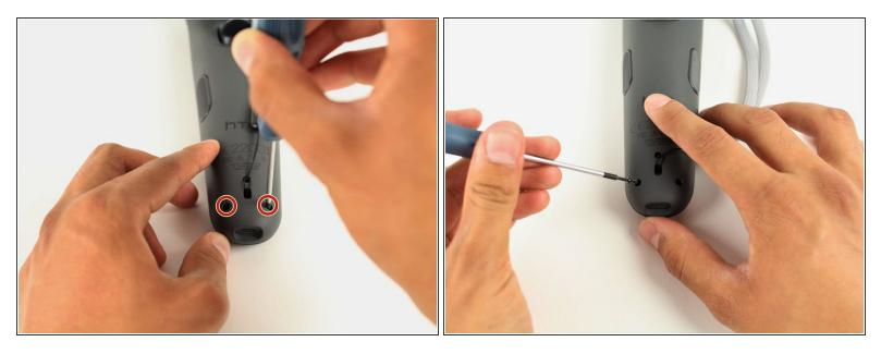
• Use the T5 Torx screwdriver to remove the two black 5.2mm screws on the back gray panel.
