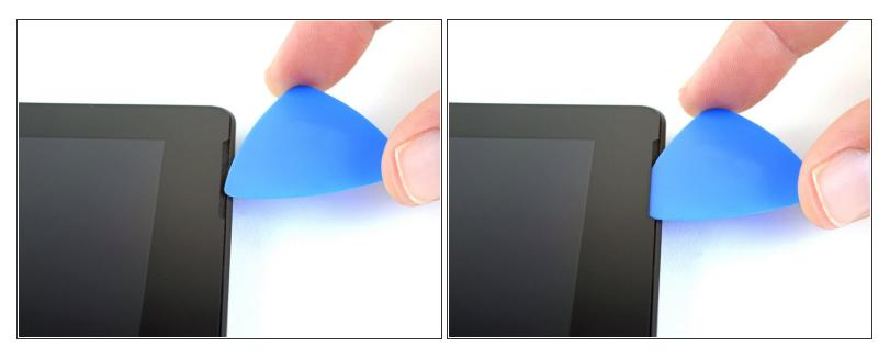
Insert an opening pick into the speaker opening on the screen and slide the pick under the glass.
