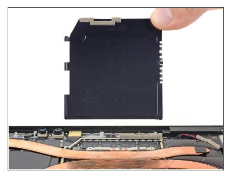
• Remove the heat sink shield.
