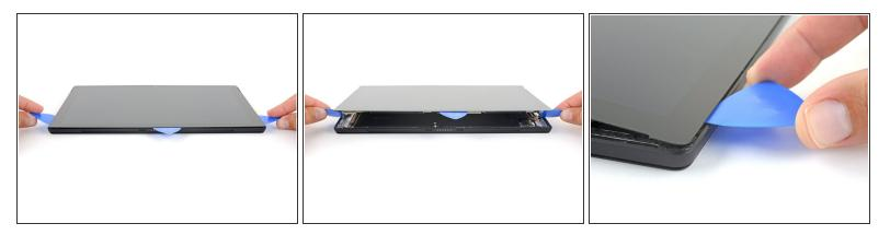
Very slowly lift the screen assembly away from the Surface case. If you encounter any resistance, stop and check that all the adhesive is separated.
