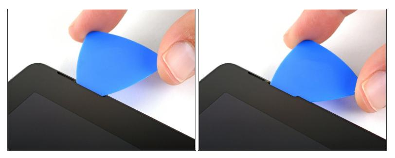
Rotate the pick toward the bottom of the Surface to slide it underneath the lower edge of the speaker cutout.
