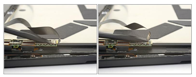
Use the flat end of a spudger to pry the display interconnect cable straight up and out of its socket on the board.
