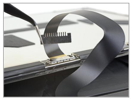
• Pull the rest of the shield off of the digitizer connector and remove it.
