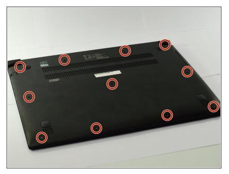
With the laptop upside-down, remove all 11 M2 x 6.0mm screws from the cover plate using the Phillips #0 screwdriver.
