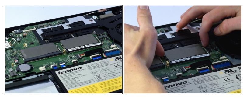
• Release clips on both sides of ram unit.
